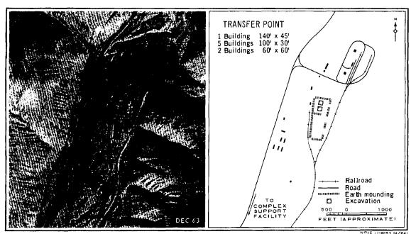
FIGURE 4. RAIL-TO-ROAD TRANSFER POINT.
